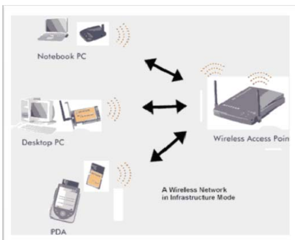
Fig. 1: Infrastructured Wireless Networks
